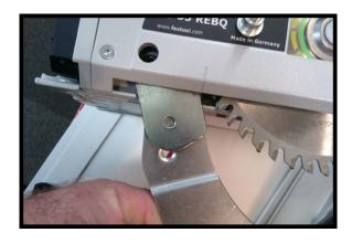
It's important that the hole in the riving knife on the saw lines up exactly with the hole on the CMS riving knife.
