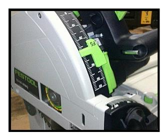
installation of the new CMS riving knife in the TS55R saw. In the previous version you had to activate the Fast Fix blade changing mechanism, unscrew the plunge cut riving knife and replace it with the CMS riving knife.
