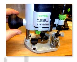
The zero point on the measuring scale represents the top surface of the workpiece so our next step is to set the overall depth of the cut, or where we want the bottom of our trench to be.
