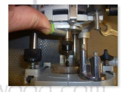
Step 3: Whilst still depressing the spindle lock, insert the router cutter in the collet. Insert
