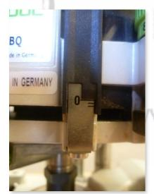
With the plunge lock still set, rotate the depth turret until the shortest turret, ("c" in the photo above), is directly below the guide bar, then loosen the guide bar lock so that the guide bar rests on the top of turret (c).
