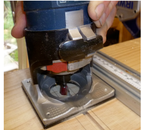
Cutting the dovetail trench
