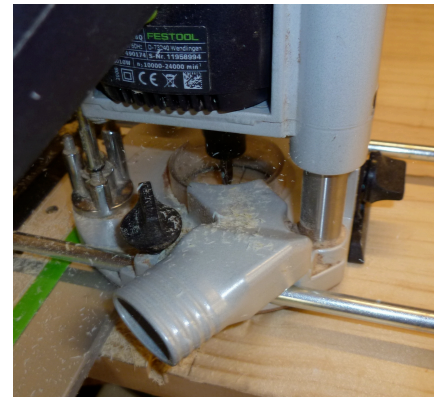
Cutting the straight trench
