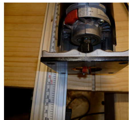
Dovetail cutter at 6mm
