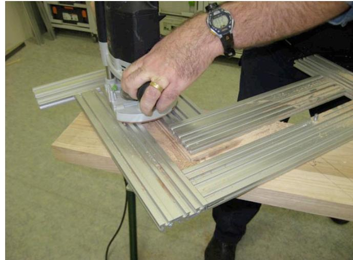
When the first stringer is complete, place the 2<sup>nd</sup> stringer on the workbench and line up the MFS.
