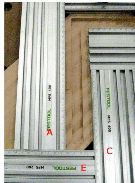
To set the length of cut of the riser, use the trammel pins that come with the MFS as stops to limit the travel of the router
