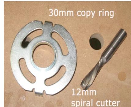
Our first step is to calculate the offset between the router cutter and the copy ring
