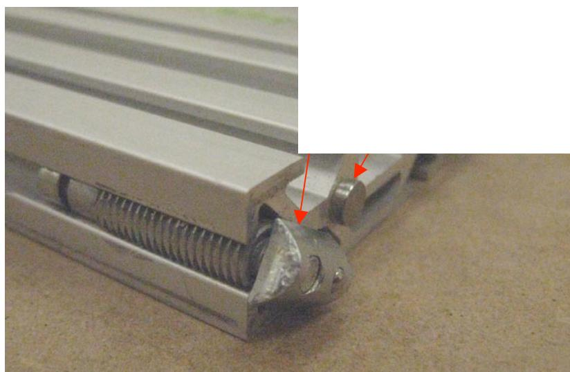
When connecting two sections together place the two pins in the opposing channel then insert the 1/2 round dowel with the ball bearing end in first. When fully inserted tighten the screw.
