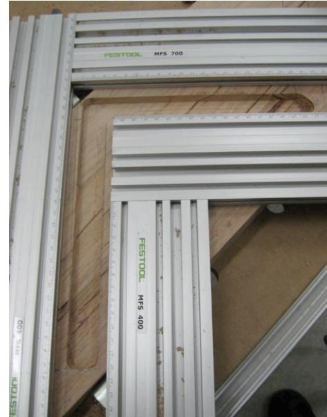
The beauty of the MFS system is that once you've cut your first set of tread and riser channels, you can simply slide the MFK along the stringer using the L brackets as guides
